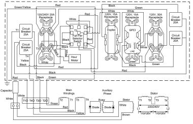
Figure 32 - Wiring Diagram, Models RGH5500A
